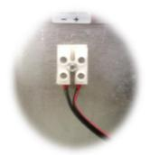
Power supply cables from the power supply are to be connected directly to the power connector of the control electronics or to the terminal block **X1** in the turnstile (see the figure).
