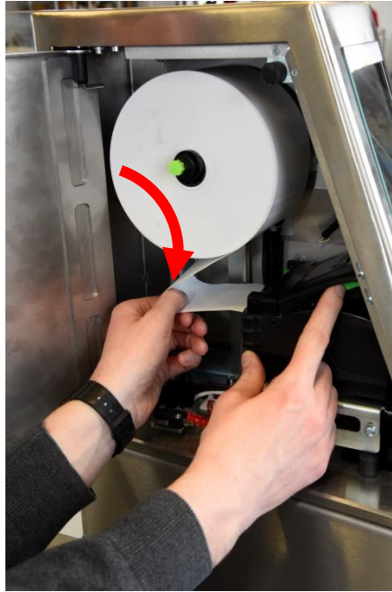
Figure 12: Releasing the top cover of the printer and pulling out the paper
