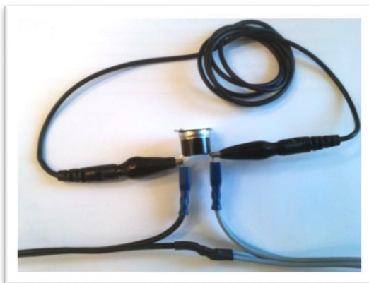
bridging the thermostat - version 1
