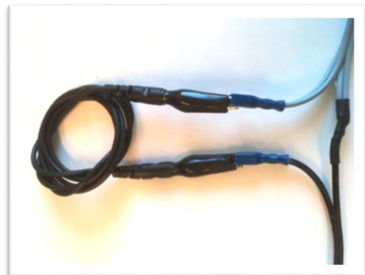
bridging the thermostat - version 2
