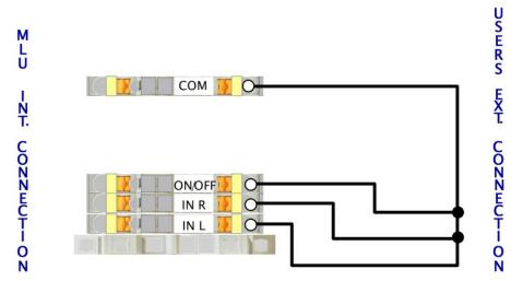
The control signals are connected to the X2 terminal.
