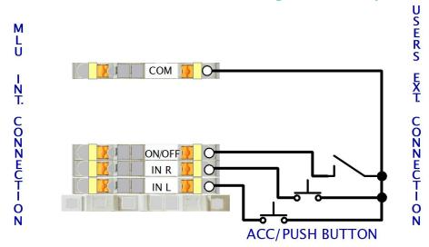
The control signals are connected to the X2 terminal.
