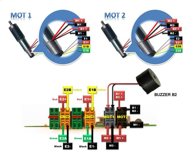
The power supply of motor drive units is realized by a pair of thicker cables of red and black colour (M1 +, M1-), or (M2 +, M2 -), coming out from the middle part of the motor drive unit. Motor 1 (MASTER) is connected directly to the MOT2 connector. Motor 2 (SLAVE), which is located in the second half of the turnstile passage gate, is connected to the MOT1 connector through respective terminals of the X2 and X3 terminal blocks.
