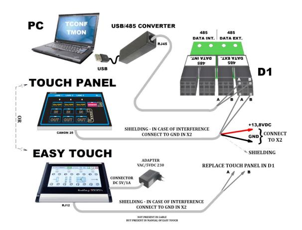
DATA EXT. serves for PC connection via RS485-USB or RS485 Ethernet and also for connection of control panel (Touch Panel / Easy Touch).
