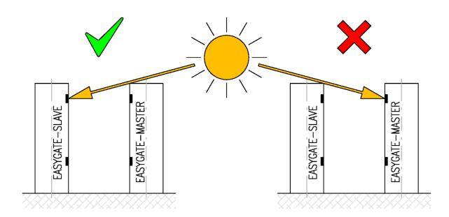
If it is not possible to carry out appropriate measures or turn the installation, we must substitute the transmitting and receiving optical sensors of the respective passage gate. In case such substitution is performed, it is necessary to expect that the turnstile will be put out of operation for about 3 hours. If you are about to make such a substitution, please request a separate Manual for the respective turnstile type.
