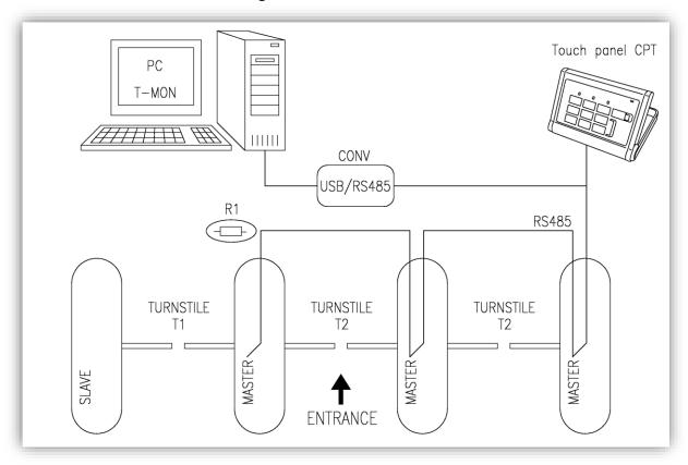
The connection of PC, Touch panel and turnstiles via the RS485 line is shown of the figure.
