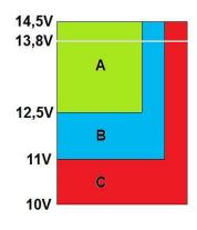
14.5VDC Absolute maximum of power supply voltage - normal device functioning without limitations (this limit must not be exceeded).
