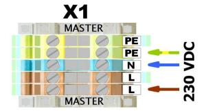
Connection of supply voltage in case of using the **230VAC** mains supply.
