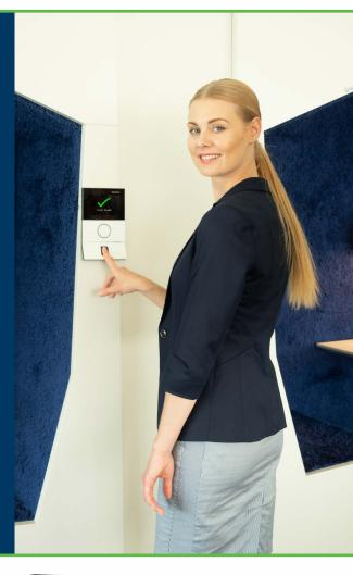
The GT7 terminal, available with and without fingerprint sensor, impresses with highlights including identification via RFID, NFC, or wireless interface, and the unique app concept that is uploaded to the universal hardware.
